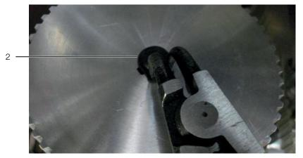
Fig. 10: Remove the circlip
